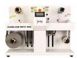
A compact tabletop model with many of the features of a professional digital die-cutting machine: laminating, die-cutting, die extraction, slitting and rewinding. Thanks to its infinitely variable servomotor and sturdy construction, you can achieve high cutting precision and perfect results. The maximum media width is 240 mm, enabling production of labels up to 230x300mm.
