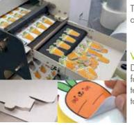
The machine's web control guide provides precise track alignment for 🌌 a perfect finish. Rolls that were initially wound incorrectly on the digital press can be corrected. This saves time and waste.
