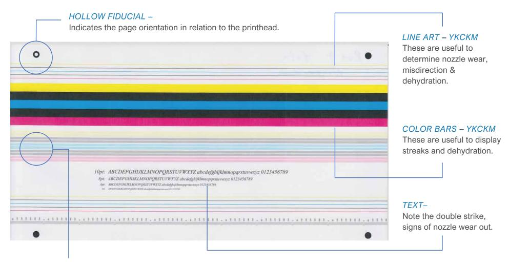
YKCKM NOZZLE PATTERNS – very good for assessing dot placement, overall nozzle health, wear and random contamination & non-ejecting nozzles.
